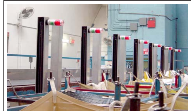
Items are counted and collected directly into slings. An alarm indicates when the sling is full.
